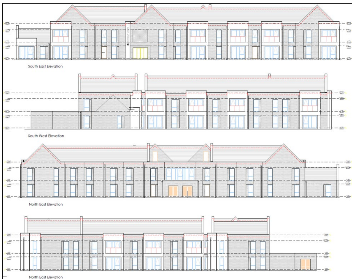
Figure 9: Building elevations showing proposed height increase
